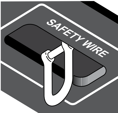
Figure 4: Safety wire attachment point
